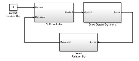
**Note:** For a more detailed analysis of a similar ABS model, see Modeling an Anti-Lock Braking System.
