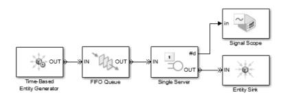
The existence of the entity path does not guarantee that any entity actually uses the path; for example, the simulation could be so short that no entities are ever generated. Even when an entity path is used, it is used only at a discrete set of times during the simulation.
